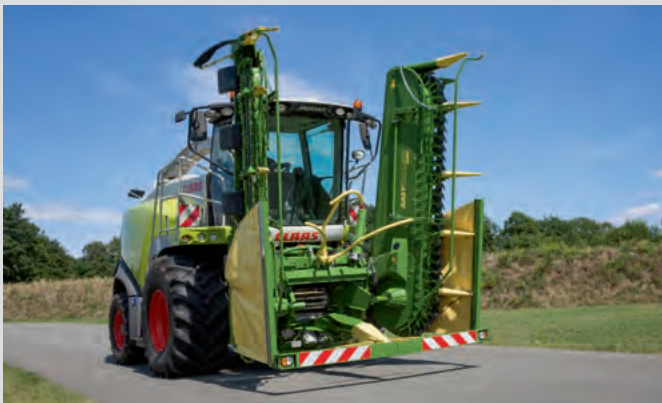
The 2-section maize header is available as a 4.5 m, 6 m and 7.5 m unit.
