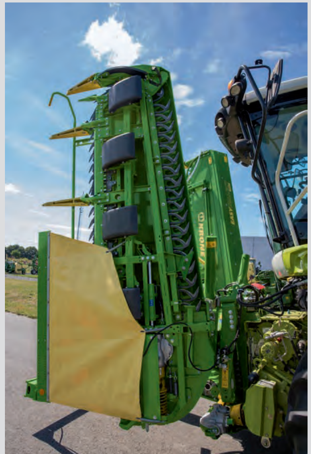
The 2-section maize header is available as a 4.5 m, 6 m and 7.5 m unit.
